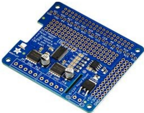
Obr. 3. Adafruit DC &amp; Stepper Motor HAT [2]
