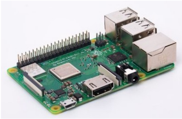
Obr. 2. Raspberry Pi 3 Model B+ [1]
